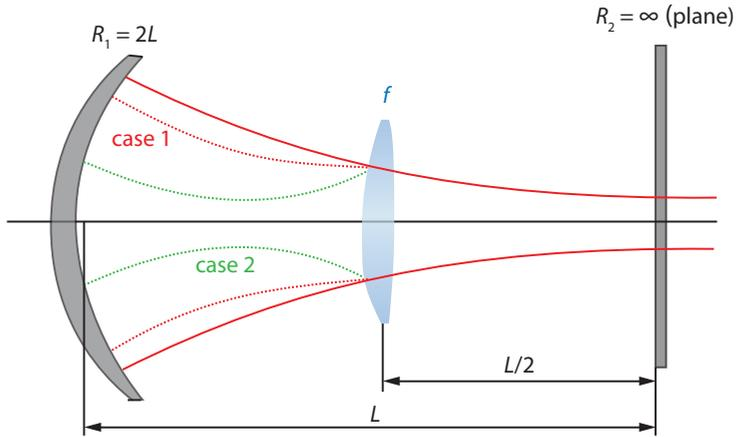
**Figure SB.9** Geometry for thermal lens inside a resonator.
