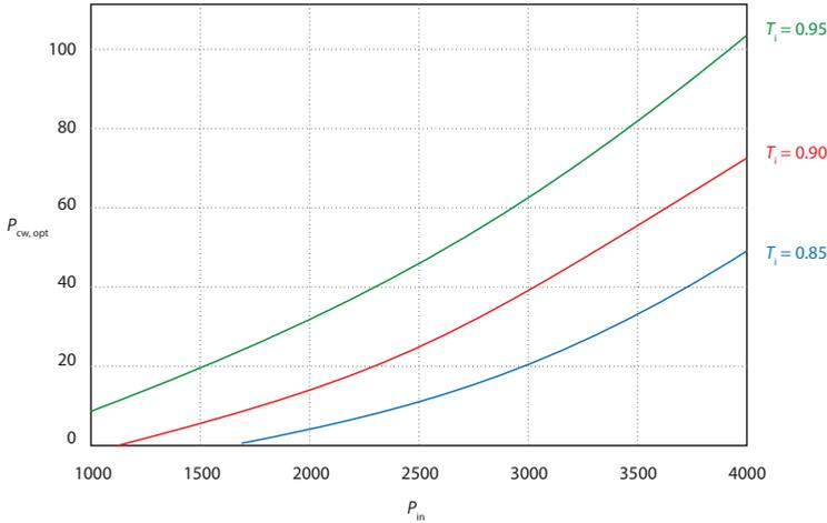
**Figure SB.7** Maximum cw power for various internal losses as a function of the pumping power.
