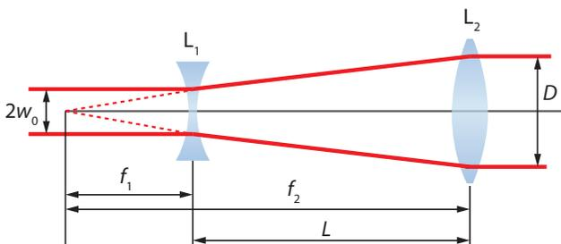
**Figure SB.1** Ray diagram of a Galilei telescope.
