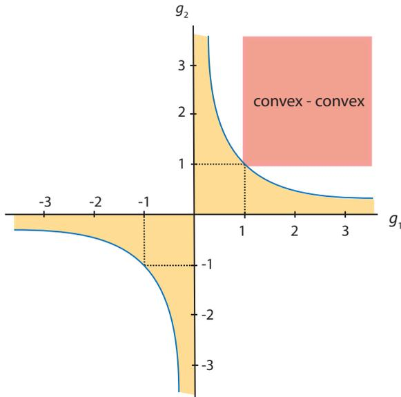
Figure SB.8 Stability diagram for convex-convex laser resonators.
