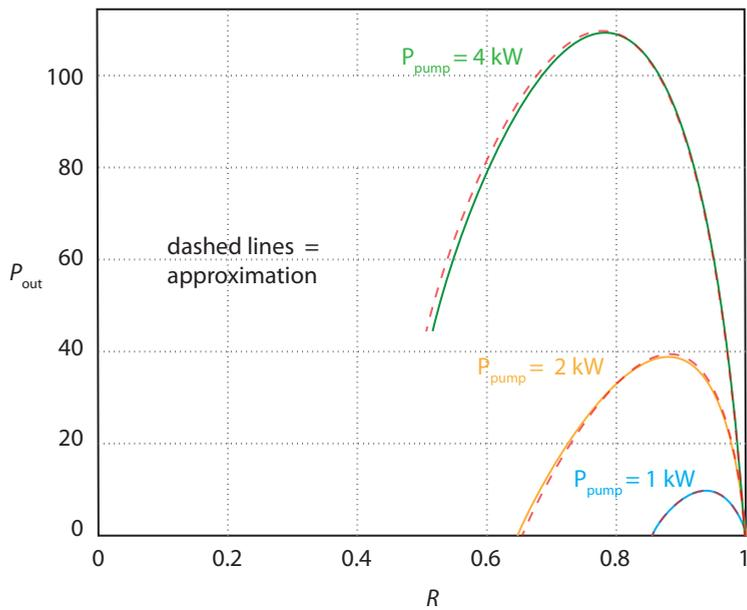
**Figure SB.6** Output cw powers for various pump powers as a function of the outcoupler reflectance. Comparison of exact solution (solid line) and approximation (dashed line).
