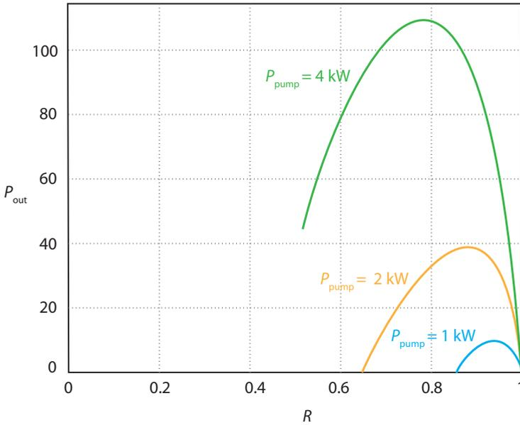
**Figure SB.4:** Output cw power for various pump powers as a function of the outcoupler reflectance.
