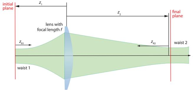
**Figure SB.3** Gauss beam transformation by a focusing lens.
