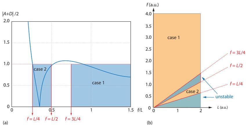
**Figure SB.10** Stability condition and areas for a resonator with length  $L$  and in the presence of a thermal lens with focal length  $f$ .
