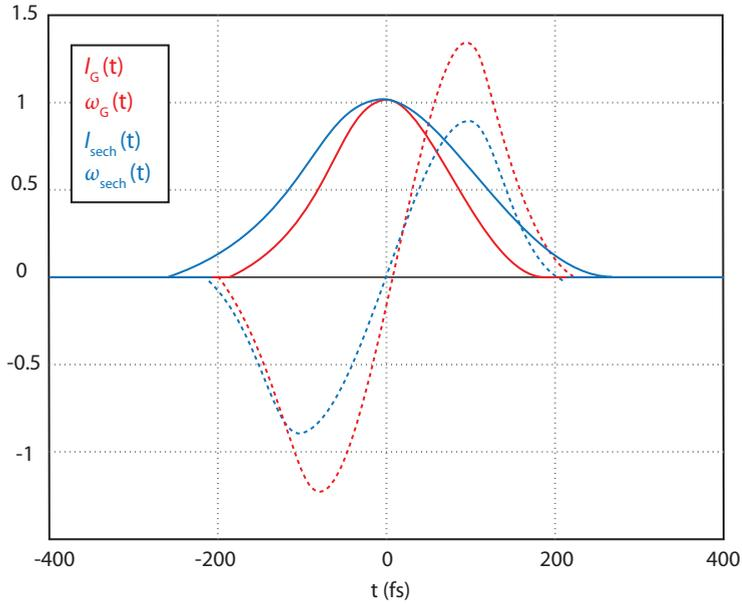
**Figure SB.12** Pulse envelope and frequency chirp in a Gaussian and a  $\text{sech}^2$  pulse in a nonlinear medium.
